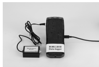
a pressure sensor connected to a datalogger 連接至數據記錄器 (datalogger) 的壓力感應器 (pressure sensor)
